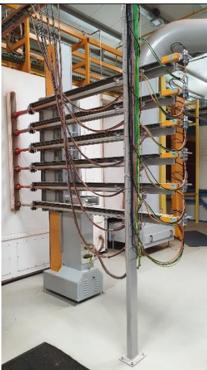
Fig. 8: Servo motors on all pistols for horizontal positioning to the optimum distance towards colored piece
