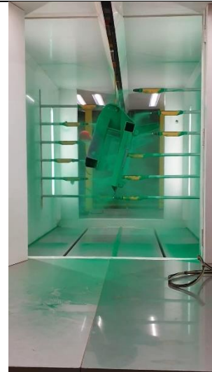
Fig. 7: Automated powder painting pistols with horizontal servo movement
