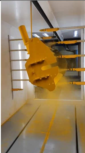
Fig. 6: Automated powder painting pistols with horizontal servo movement
