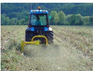
Hammers as standard, Y knives as option for lightweight tasks.
