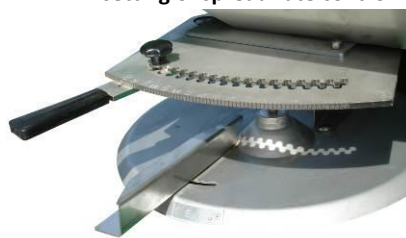
INOX spreading disc with adjustable vanes
