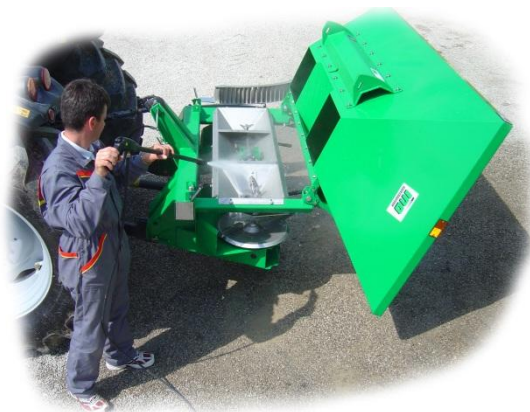
Overturnable hopper - easy cleaning & maintenance
